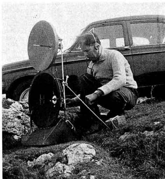
Last month we reported an 80-mile record QSO on 13cm made by G3IUD/P and G3NLZ/P. G3NLZ, who accompanied G3IUD to the Great Orme, North Wales, took several photos of the set-up, this one showing Mike, G3IUD aligning the dishes. Everything had to be securely anchored with string and stones to counteract the effect of the usual high winds experienced on the Great Orme.
